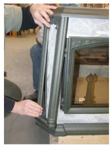
3. The tie rods are fastened with a ½" hex nut, which is located close to the leg bolts. Now lift upward on the large top frame just above the first of the cast corners and
